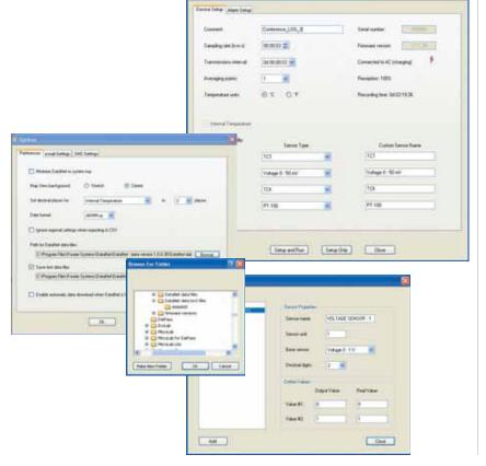
Ability to define custom sensors based on current, voltage and pulse inputs
