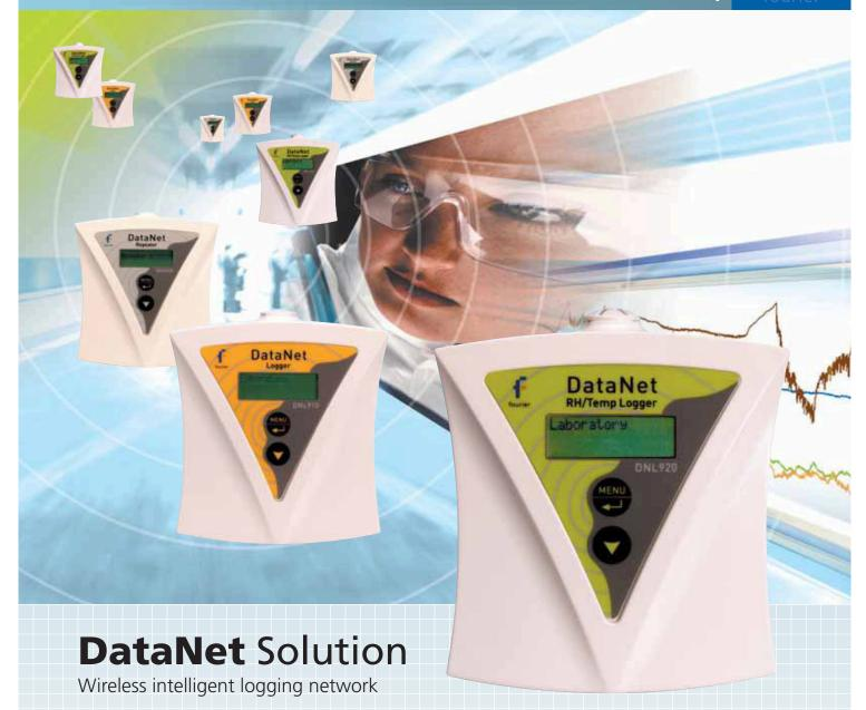
DataNet is a multi-unit data acquisition system. Data transmission from end units to the central computer utilizes the ZigBee wireless telemetry protocol. DataNet data loggers feature 16-bit resolution, with four external channels supporting direct measurement and recording of PT-100, thermocouple, voltage, current, dry contact, frequency and pulse. Internal sensors include temperature and humidity.
